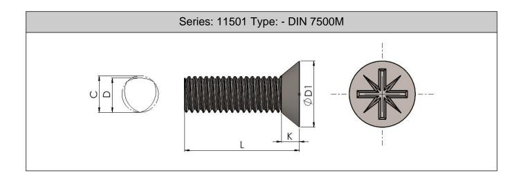
Thread forming screws have a trilobular thread form. These require a low level of assembly torque to initiate thread forming in sheet metal, castings and alloys. Further benefits: Screws form a female thread capable of accepting a standard metric machine screw should the need arise. The three lobed thread design allows the displaced parent material to cold flow into the relief areas of the screw thereby increasing the resistance to vibration and loosening of the screw.
