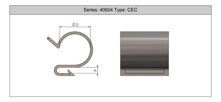
**Cable Edge Clips** removed without removal of the clip makes them very useful where service is required. Material: Spring Steel Finish: Black Phosphate or Trivalent Zinc
