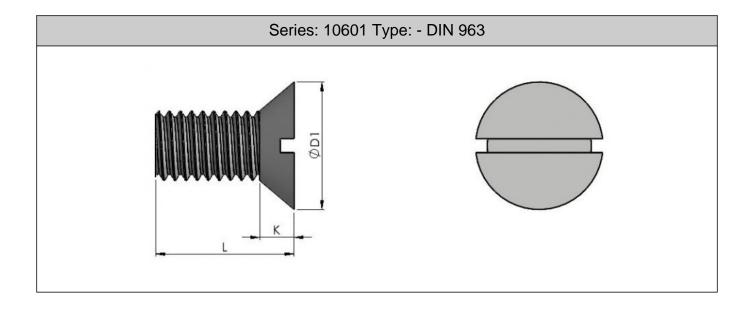
Steel - Zinc Clear - 60Stainless Steel A2 - Self Colour - SSStainless Steel A4 -Self Colour - A4 To get the part number replace \*\* with the length found in the tables below followed by the finish code:
