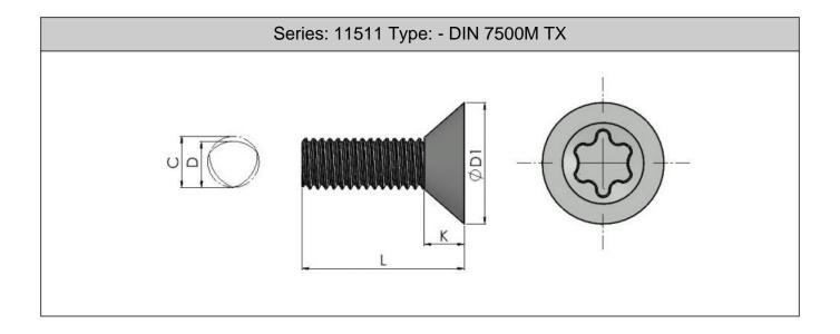
Thread forming screws have a trilobular thread form. These require a low level of assembly torque to initiate thread forming in sheet metal, castings and alloys. Further benefits: Screws form a female thread capable of accepting a standard metric machine screw should the need arise. The three lobed thread design allows the displaced parent material to cold flow into the relief areas of the screw thereby increasing the resistance to vibration and loosening of the screw.
