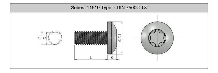
form a female thread capable of accepting a standard metric machine screw should the need arise. The three lobed thread design allows the displaced parent material to cold flow into the relief areas of the screw thereby increasing the resistance to vibration and loosening of the screw.
