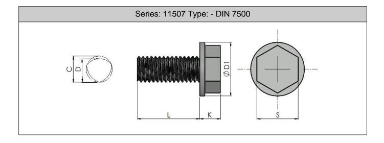
arise. The three lobed thread design allows the displaced parent material to cold flow into the relief areas of the screw thereby increasing the resistance to vibration and loosening of the screw.
