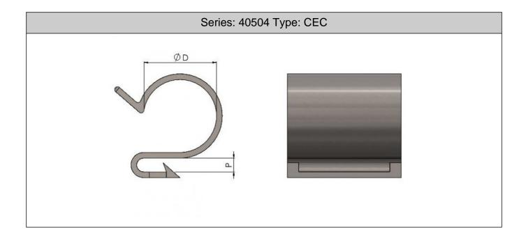
removed without removal of the clip makes them very useful where service is required. Material: Spring Steel Finish: Black Phosphate or Trivalent Zinc
